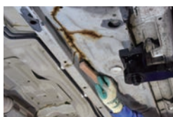
① Remove rust to some extent with a wire brush.
