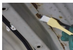
② Apply rust conversion agent with a brush. ※ Wash with water after using the brush.
