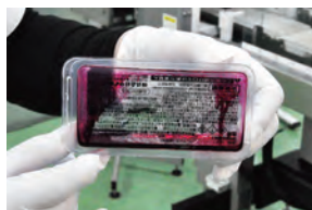
Crack detection test at heat seal package.
